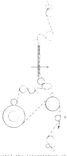
Before threading turn the motor knob until the intermittent stops and add an additional half turn. (Motor knob)
