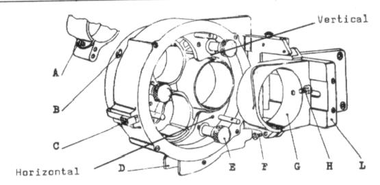
This lens turret is standard equipment on most Cinemeccanica Victoria projectors. It has been designed to mount one lens having a diameter of 70.6mm. (2 25/32") and two lenses having diameters of 62.5mm.(2 7/16"). Both diameter lenses are available from CARBONS, INC. A special adapter, part number 10-661K, is also available to permit mounting of some standard 70.6mm. lenses in the smaller mounts by placing the adapter over the 53.5 diameter section of the lens.
