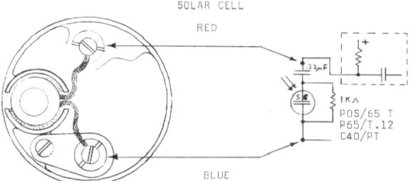
NOTE: The POS/65T preamplifier and C40/PT amplifier have the negative side of the supply connected to ground. The P/65 T.12 preamplifier has the positive connected to ground. Thus, it is necessary to follow the photodectors wiring instructions according to the different couplings. Regardless of type cell, both leads are above ground on all projectors now being supplied.
